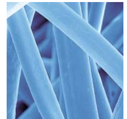
Separet filter medium unloaded, magnified 200 times
