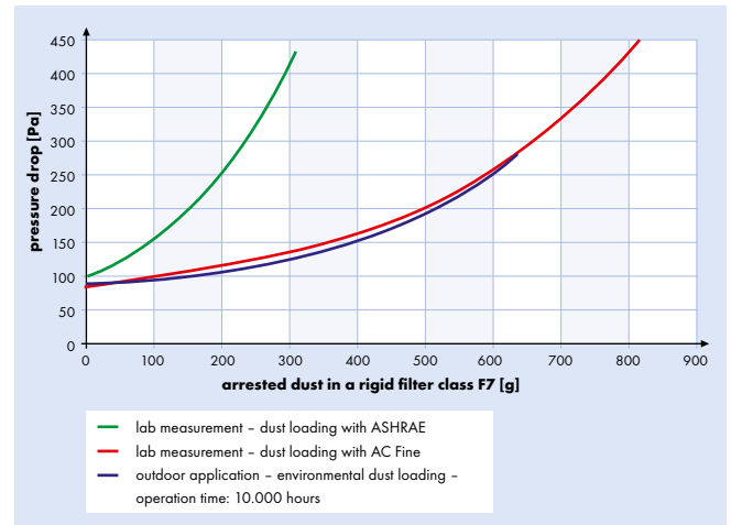
Figure 1: Comparison of pressure drop behaviour for a rigid filter class F7 with AC Fine, ASHRAE and environmental dust loading at 3400 \text{m}^3/\text{h}
